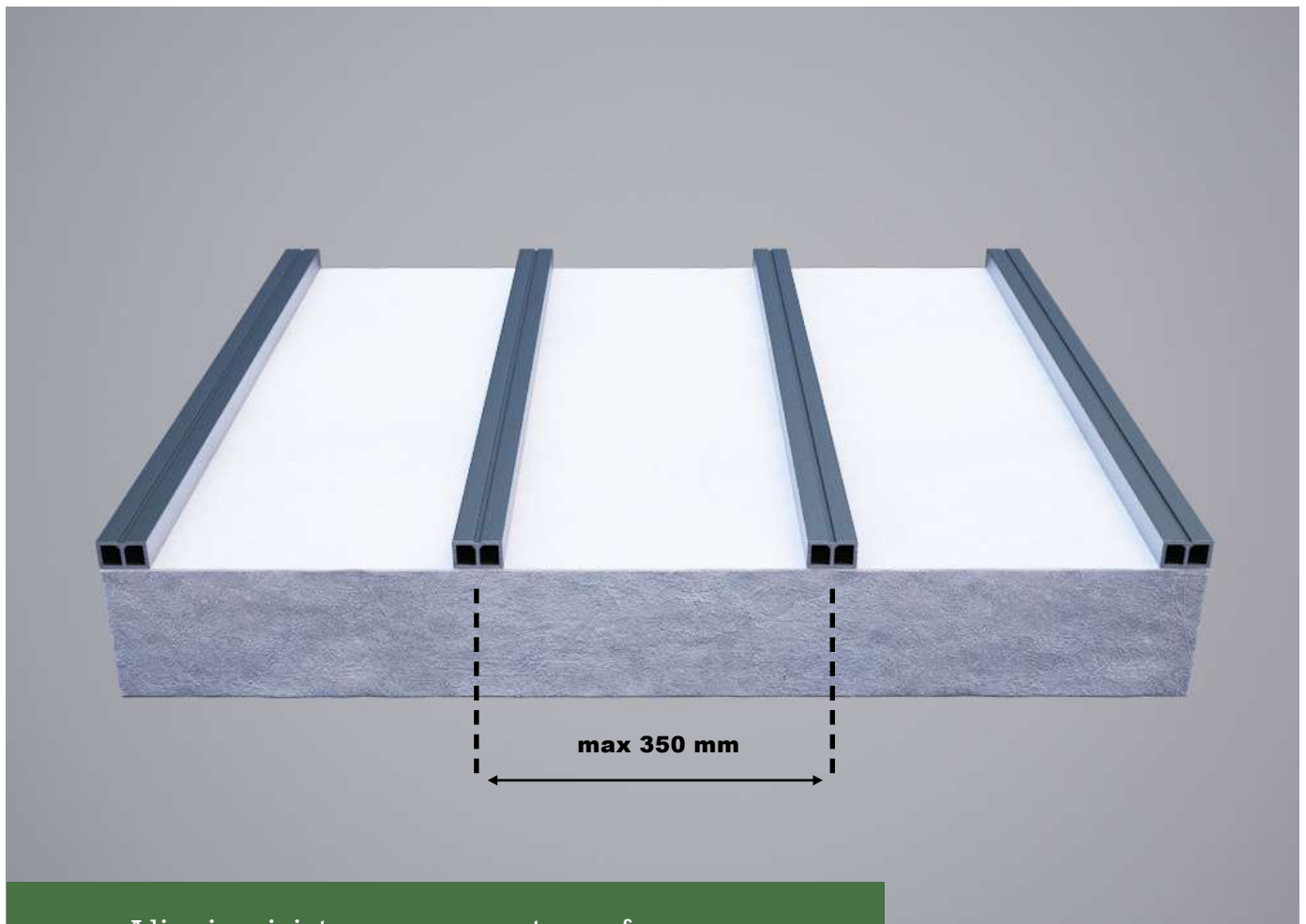
Aligning joists on a concrete surface
